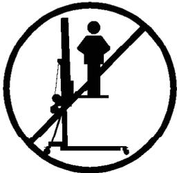
**3.1** - The TE-074 is a machine designed to elevate loads upwards in a vertical direction, It should NEVER be used as a platform to elevate people.
