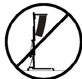
**3.4** - This lift should NEVER be used to elevate a load that has not been properly checked. It is necessary to verify that the load is correctly supported and centred on the appropriate lift support so that the weight of the load will only elevate in a vertical direction.
