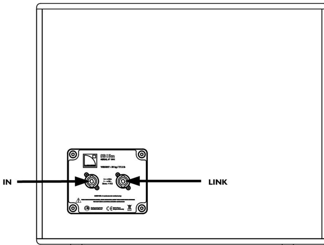
The SBI 5m subwoofer is equipped with two 4-point SpeakON® connectors.
