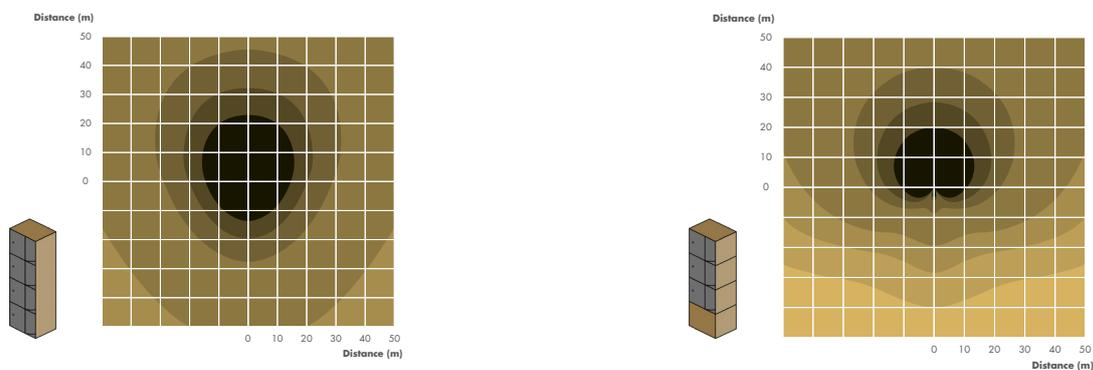
► SPL mapping of a block of four KS21 in standard (left) and cardioid (right) arrangements, using surfaces of equal sound pressure with three dB step colored scale.
