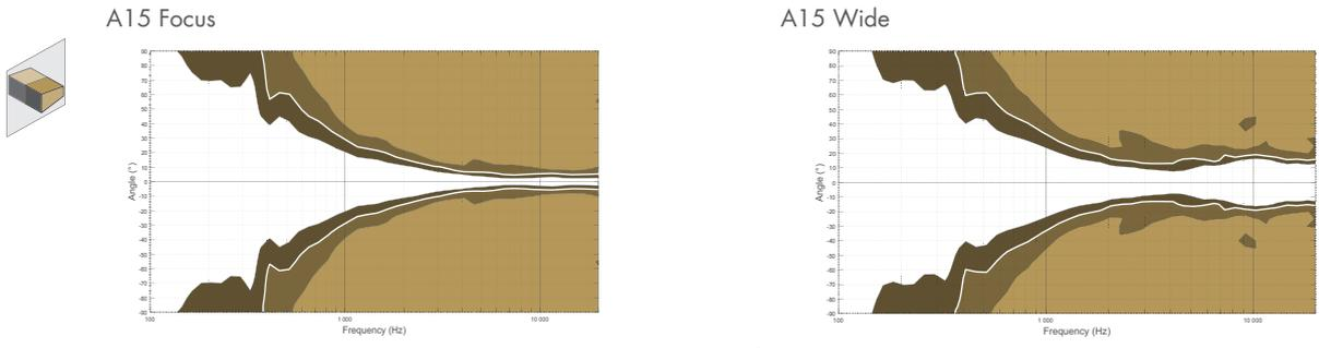
► Dispersion angle diagram of a single A15 Focus (left) and A15 Wide (right) in the vertical plane using lines of equal sound pressure at -3 dB, -6 dB, -12 dB.
