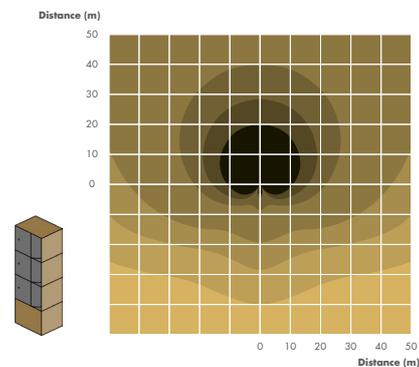
► SPL mapping of a block of four KS21 in standard (left) and cardioid (right) arrangements, using surfaces of equal sound pressure with three dB step colored scale.
