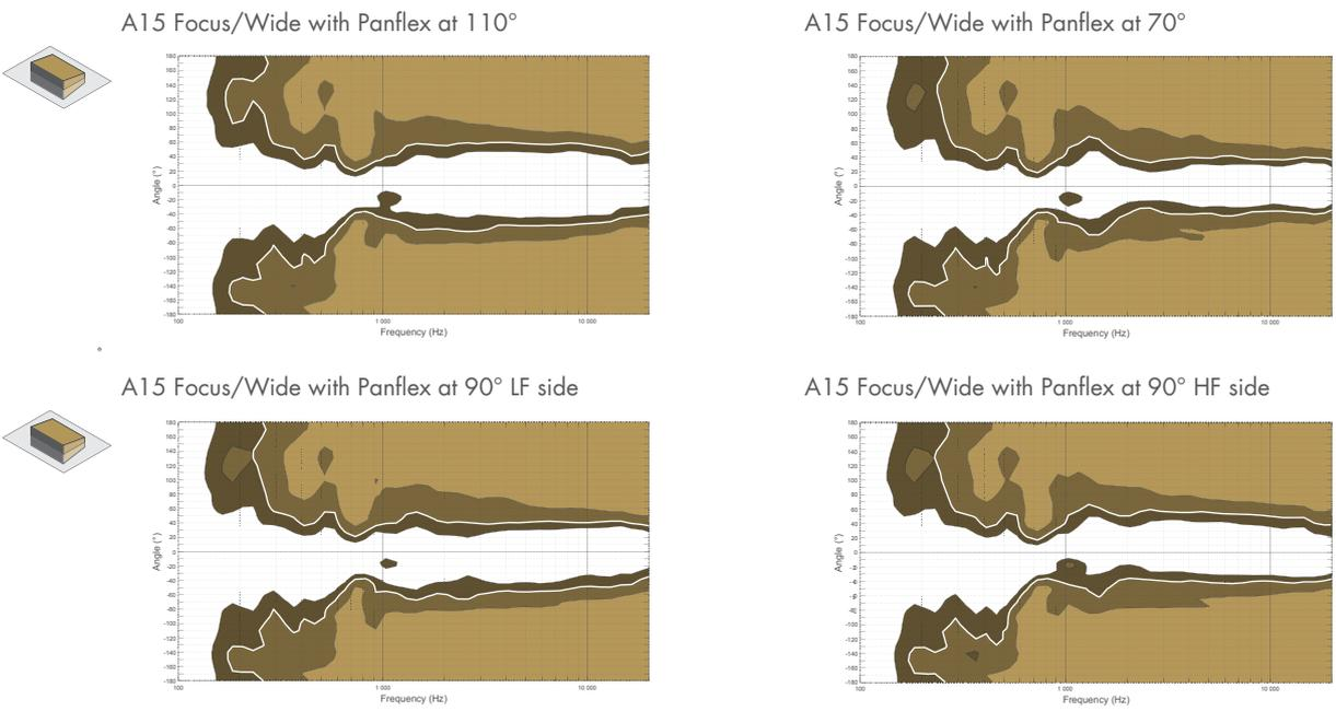
► Dispersion angle diagrams of a single A15 in the horizontal plane for all Panflex settings using lines of equal sound pressure at -3 dB, -6 dB, -12 dB.
