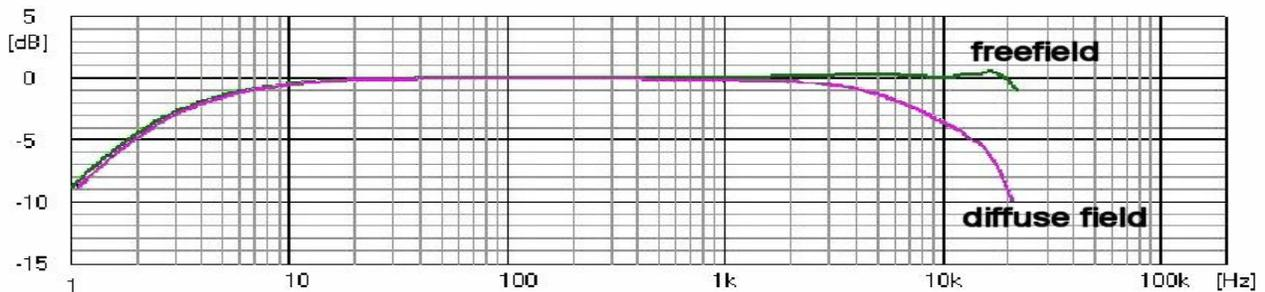
The diffuse field response is not easy to measure, because it is not easy to generate a truly diffuse sound field over a wide frequency range but there is a known procedure to estimate the diffuse frequency behavior of a free field microphone. From literature we know, that a microphone's random (diffuse) incidence response can be approximated by measuring the 90 deg incidence response relative to a single sound source.
