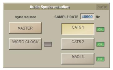
In general terms, one console should be set to Audio Sync Master and others should normally be set to derive sync from a port that is also connected to that Master console. In each of the following application examples, please pay careful attention to the required Audio Sync Settings.
